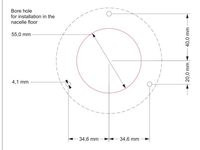
Spax screws with a diameter of 3.5 mm can be used to fix the microphone disc.
