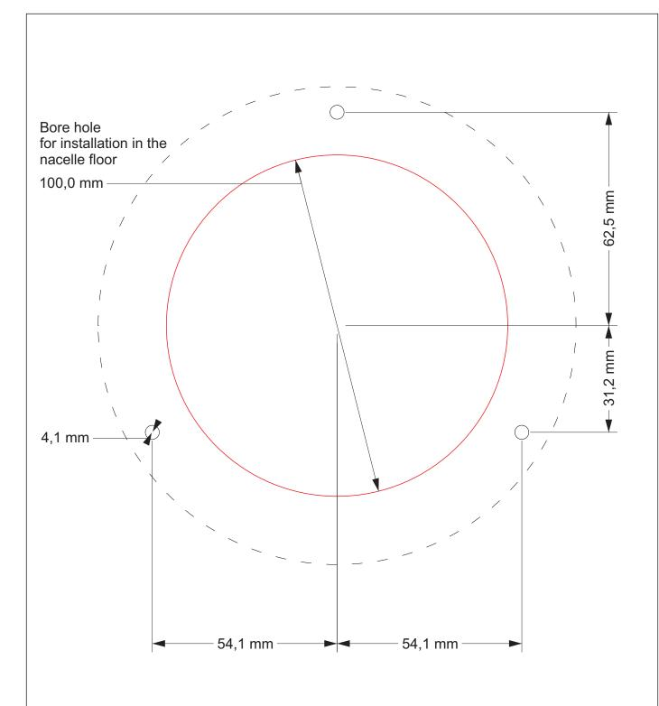
Spax screws with a diameter of 3.5 mm can be used to fix the microphone disc.
