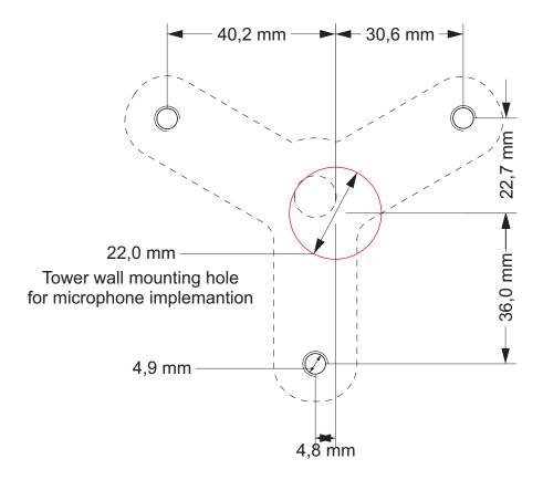
Do not place the tripod in the center of the tower wall hole, because the threaded bolt of the microphone is not radially symmetric to the microphone circumference.
