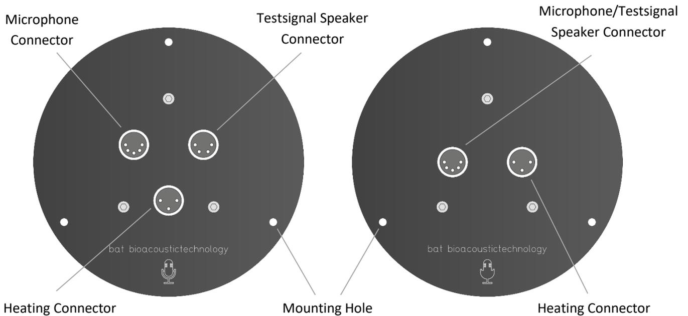
Figure 4: Old and new version of the Microphone Disc
