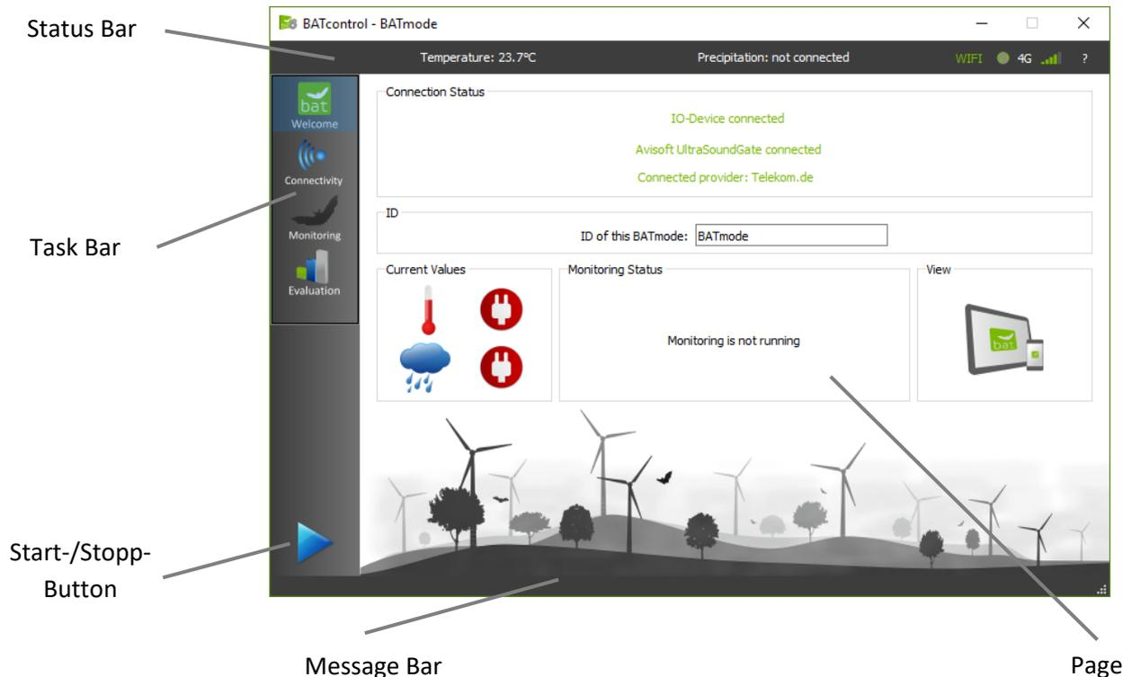
Figure 6: Structure of the BATcontrol software
