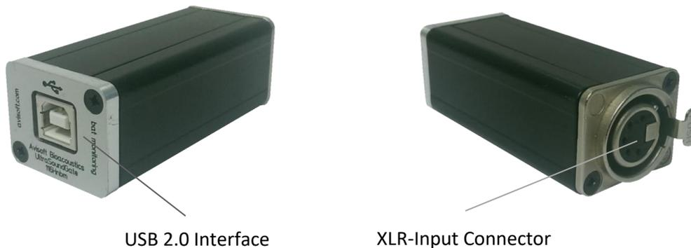
Figure 5: UltraSoundGate 116Hnbm
