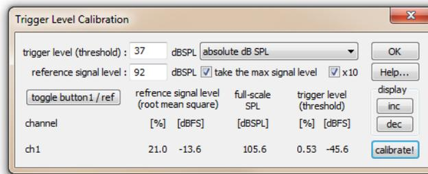
Figure 11: Trigger Level Calibration Dialog of the RECORDER Software
