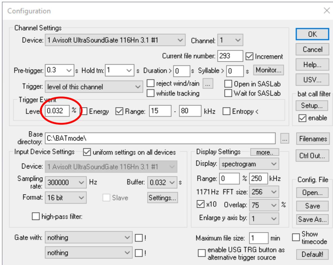
Figure 3: Configuration Dialog of the software RECORDER
