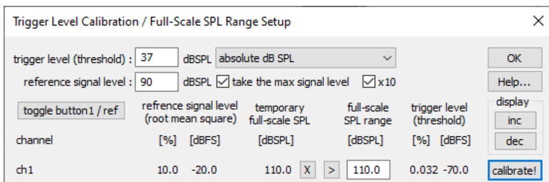
Figure 4: Trigger level Calibration dialog of the software RECORDER
